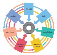
A statement about the expected tightness of the flange connection is only possible if a qualified and defined installation of the gasket has been executed.
